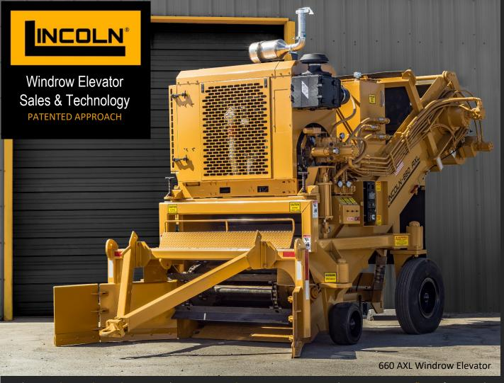
The Lincoln Windrow Elevator with our patented remixing auger provides a continuous flow of material that reblends asphalt just before entering the hopper eliminating segregation and ensuring a uniform mix temperature. Our unique product increases production and improves material handling reducing costs.
